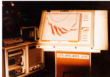
(b) The main input of UPIC was a large graphics tablet, on which waveforms and pitch data could be drawn.
