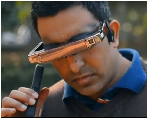
(a) A person using The vOICE integrated with a headset. The headset takes images which are converted into a soundscape and played back allowing the user to ‘see with their ears’ [32]
